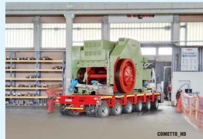
Combining Power Pack and driven axles the vehicle can become a self-propelled. Electronic control board is also available on request.
